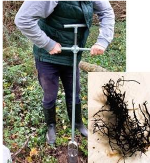
Picture (right): Sampling using the exact volume of soil for standardization of the sample. The final look of the properly sampled roots from soil cores.
