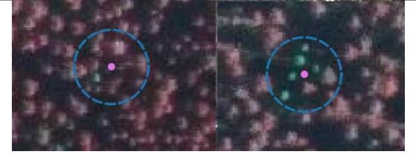
Examples of 9-m-radius field plots in North Karelia, Finland; trees appearing cyan in the image have damages caused by spruce bark beetle. The point in magenta is the plot centre point, and the blue dotted line indicates the field plot area. (Background: Aerial false colour orthophoto from National Land Survey of Finland).
