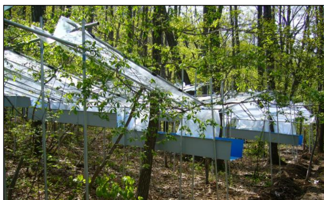
减雨控制实验样地 The experimental platform for manipulative through fall reduction
