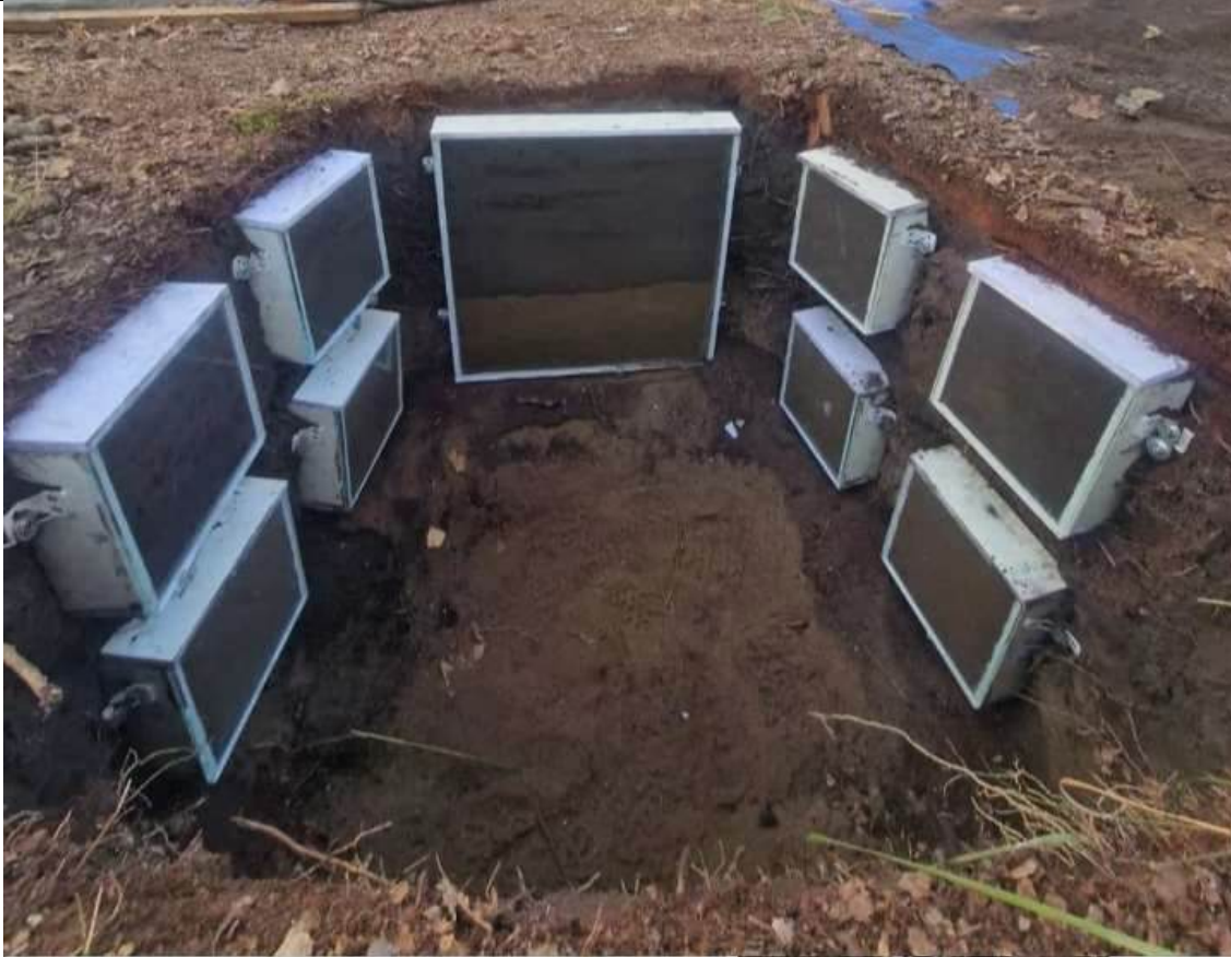
Photo of Practice Abstract 6. Rhizotrons installation at a site. Root production and mortality can be observed through the large pane of glass and smaller rhizotrons can be installed for destructive sampling of roots and soil.
